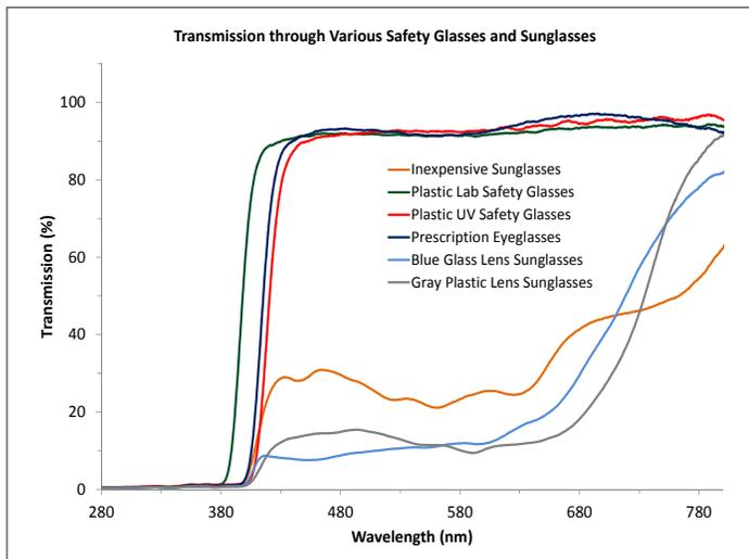
Figure 3. The Vis-NIR blocking efficiency of the more expensive eyewear options was very high, but even the least expensive glasses performed reasonably well.
