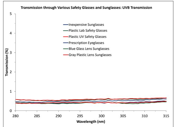
Figure 1. Regardless of lens composition, the glasses were effective in blocking UVB radiation (280-315 nm).
