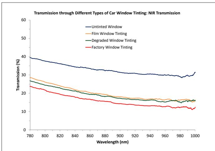
Figure 5. Effective blocking of heat-generating Vis-NIR radiation is one of the key functions of tinting in car windows.
