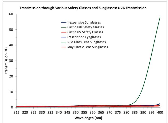
Figure 2. All eyewear samples tested demonstrated effective blocking of UVA wavelengths (315-400 nm) up to 380 nm.
