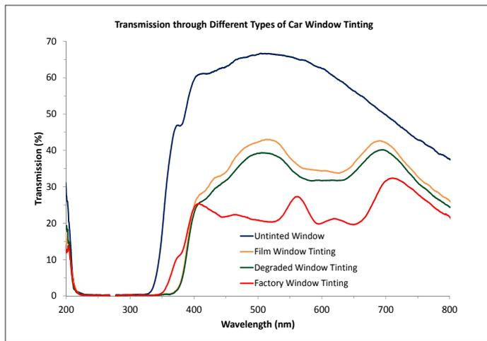
Figure 4. Factory tinting in car windows was most effective in filtering UV-Vis-NIR wavelengths when compared with other tinting options.
