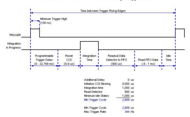
USB2000+ -- Timetable for Hardware Edge Trigger Mode
