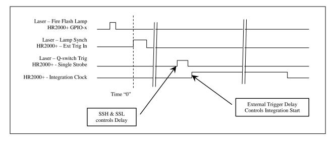
Common Clock: In order to reduce the jitter between the HR2000+'s, it is necessary to operate these on a common Clock. This is done by having the Master HR2000+ drive its Maser Clock Signal (default 2.4MHz – FPGA Register address 0), and having the other HR2000+'s use this Master Clock. This is done by configuring the master clock to drive the MCLK signal out the GPIO-1 pin (alternate function) and have the other spectrometers use this signal.
